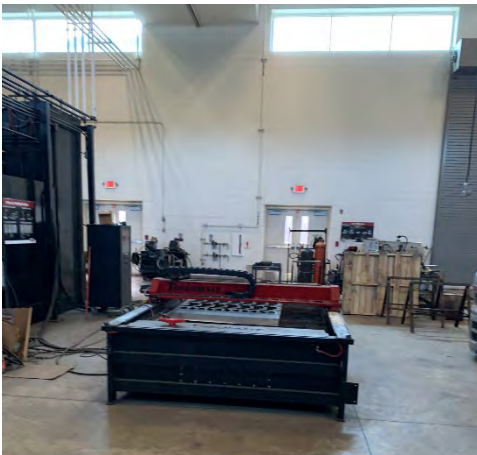
Plasma Cutter Needs an Exhaust Hood
